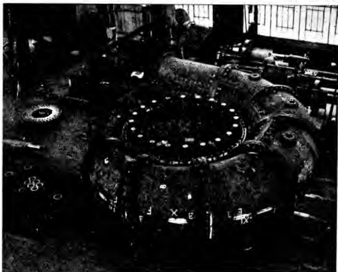
FIG. 132.—Casing for 55,000 H.P. Turbine for Queenston Plant of the Hydro-Electric Power Commission of Ontario; Showing Taylor Method of Sectionalizing.
